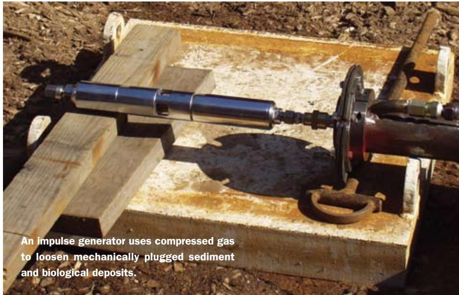
An impulse generator uses compressed gas to loosen mechanically plugged sediment and biological deposits.
